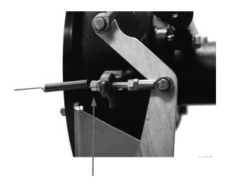
To adjust clutch linkage, loosen the two 3/8 hex nuts as shown in the picture by arrow. Check to make sure the PTO turns freely in the disengaged (handle horizontal) position. If the PTO has resistance to turning, adjust the nuts in toward the clutch fork. Check again for free play in the handle vertical position. After adjustment are made, lock the two 3/8 hex nuts together.
